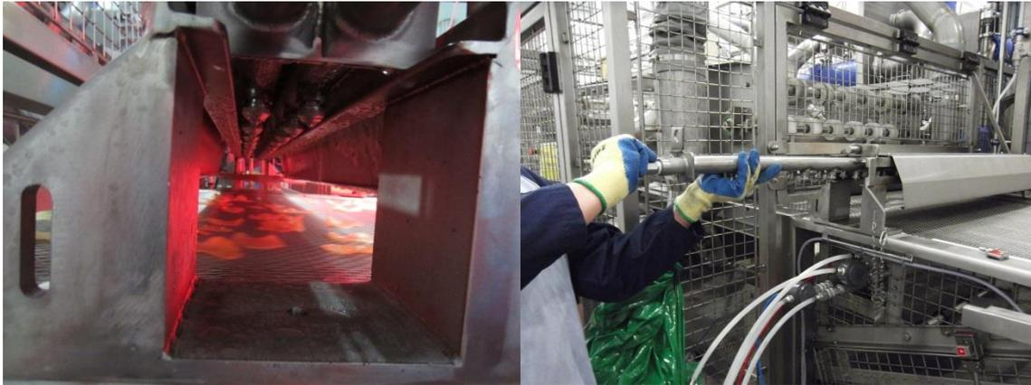
Figure 2: The spray bars on the production line (left) and the bars being removed for weekly cleaning
