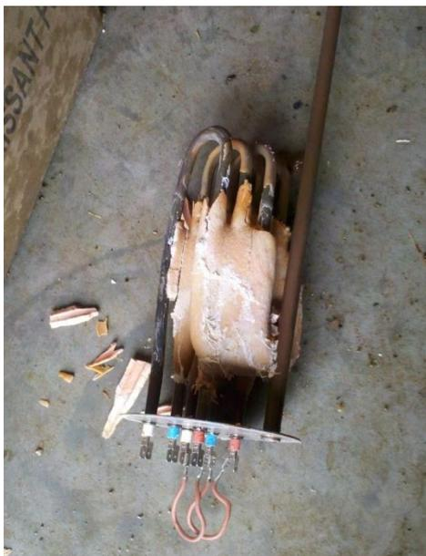
**Without HydroFLOW:** Limescale creates a strong bond between the electric heater coils. The layer is very solid and compact and can only be broken with a hammer. The heaters are unusable.
